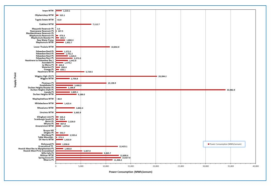
Figure 5.3 Annual Power Usage Comparison Umgeni Water Installations.
