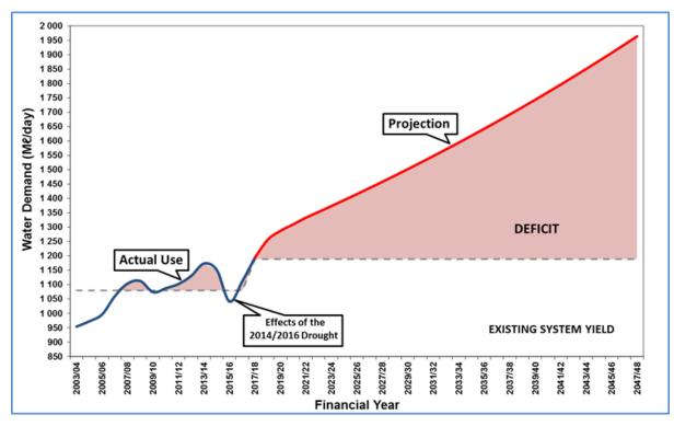
Figure 2.69 Mgeni System - Existing Water Balance
