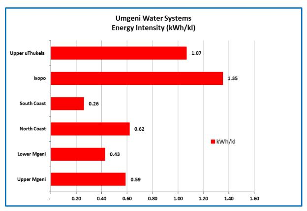
Figure 5.2 Energy requirement to supply water in Umgeni Water Systems 2018/19.
