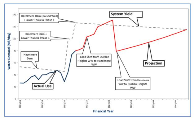
Figure 2.70 North Coast Supply System – Existing Water Balance
