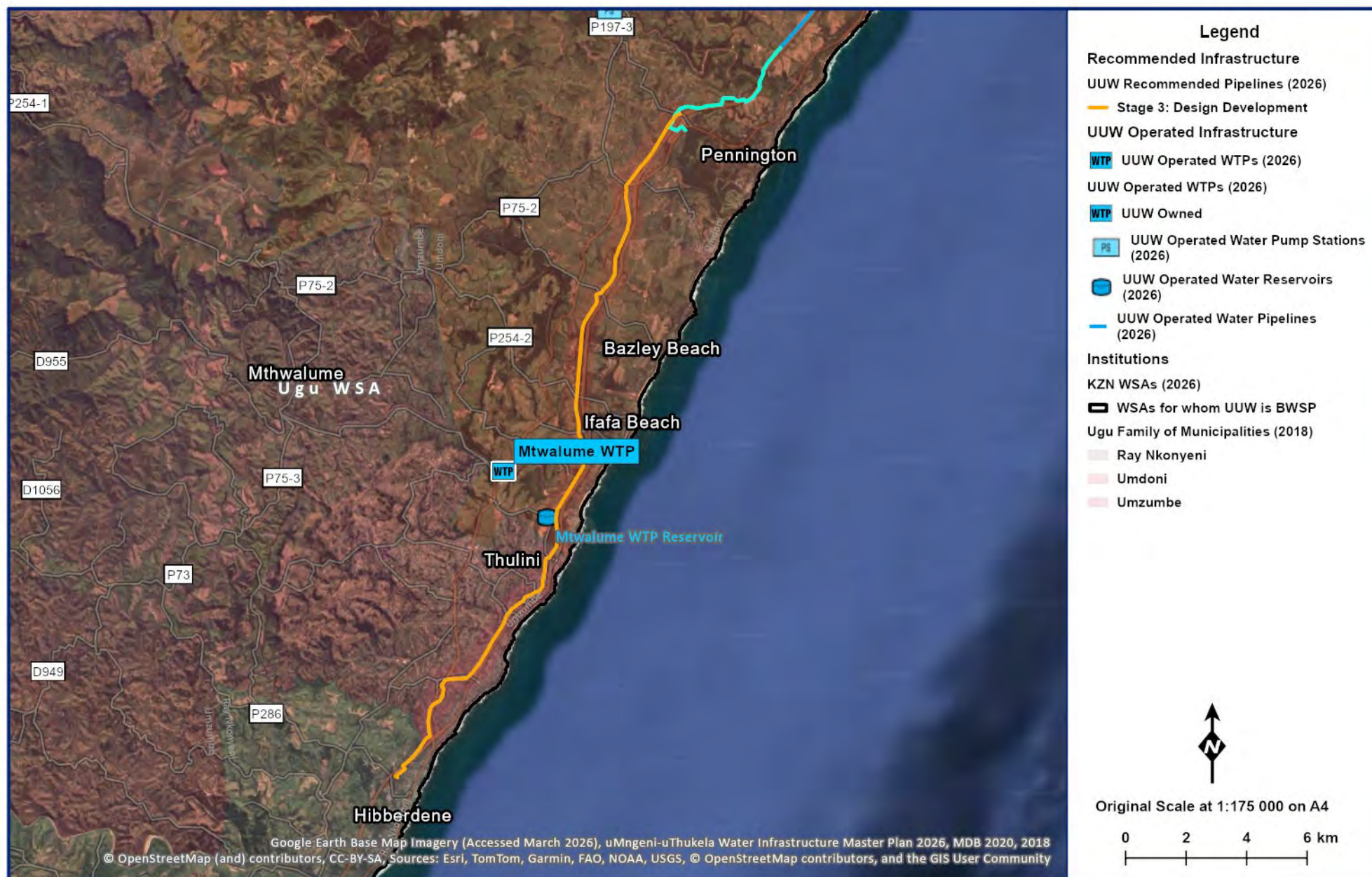
Figure 11.75 Proposed South Coast Pipeline Phase 3.
