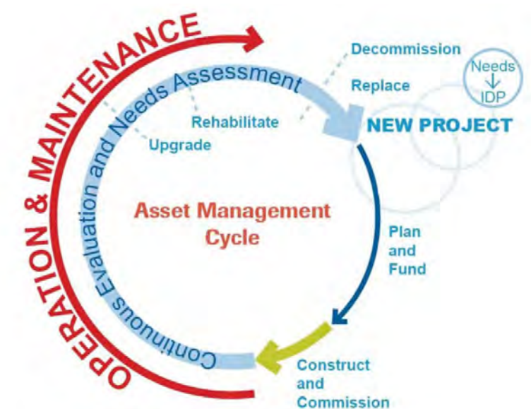
Figure 13.74 Integrated asset management (DWS 2018: 5-14).
